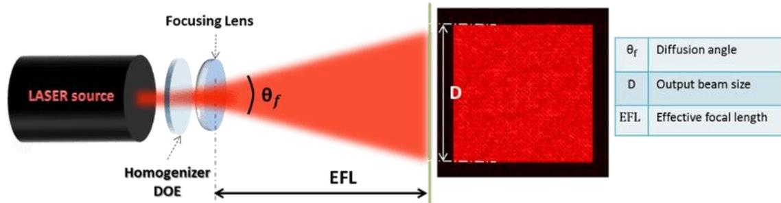
3. The optical parameters of the diffuser can be easily calculated from geometric point of view:
